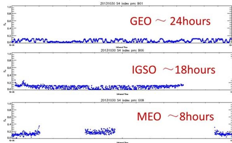
Figure 3 The lock times for COMPASS satellites
