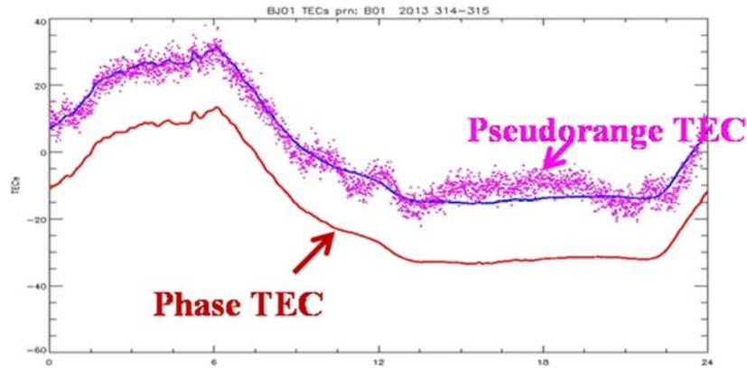
Figure 5 The TEC observations from one COMPASS GEO satellite
